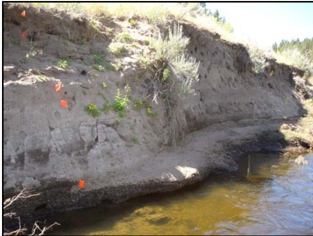
Figure B-2. Two bank profiles on the Sycan River in the project area (top) and the Teddy Powers Meadows reference reach (bottom) exhibit similar soil stratigraphy. However, the depth of pumice is substantially deeper in the project area relative to the upstream reference reach.
