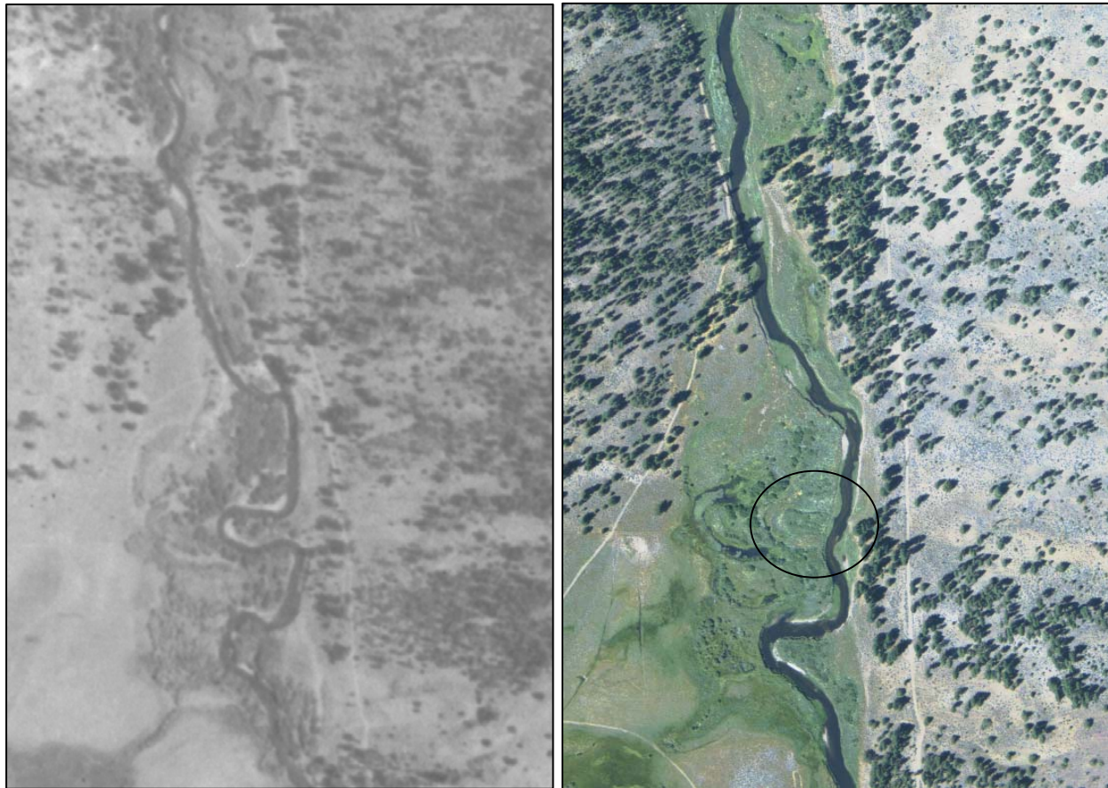
Figure B-17. A channel meander (circled) that was active in the 1941 air photo (left) was abandoned by the 1998 air photo (right). The abandoned channel segment remains apparent on the landscape although it is located above the current alignment's elevation, suggesting the channel has degraded in the reach since 1941.
