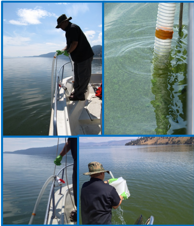
Figure 5. Klamath Tribes field crew obtaining phytoplankton samples in Upper Klamath Lake using an integrated water column sampler (tube sampler).
