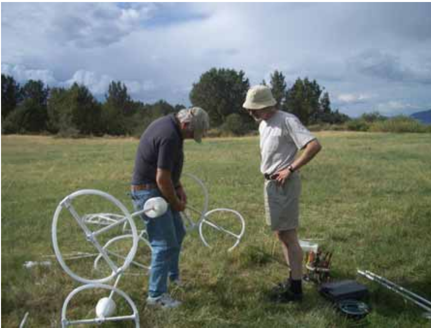
Figure 17. Assembly of spreader system for smaller enclosures on shore at Skillet Handle assay site. Note location of sliding small floats.
