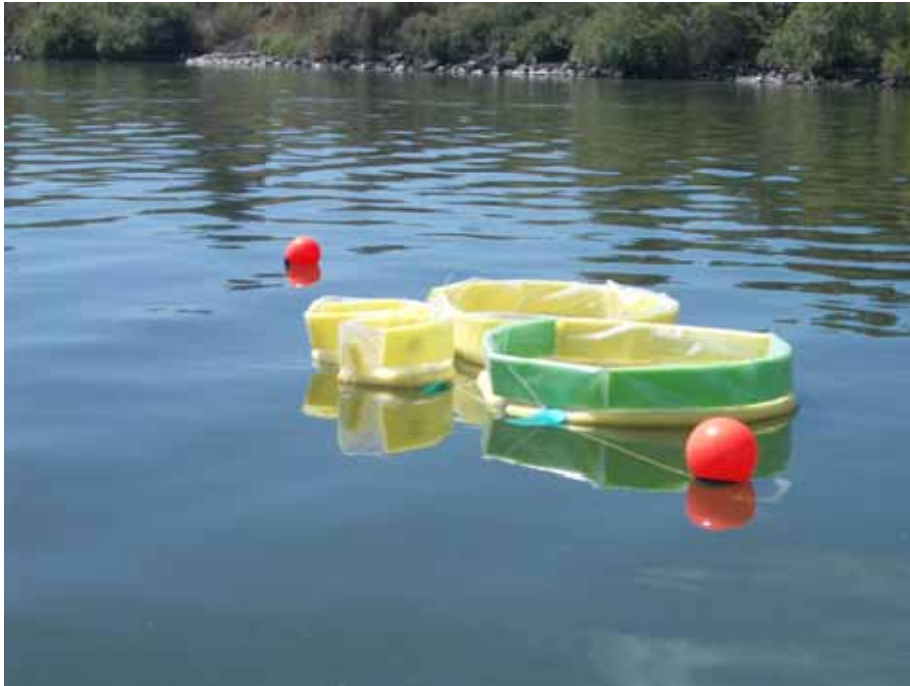
Figure 21. Array of large and small enclosures showing the freeboard created by the “noodle boards”.
