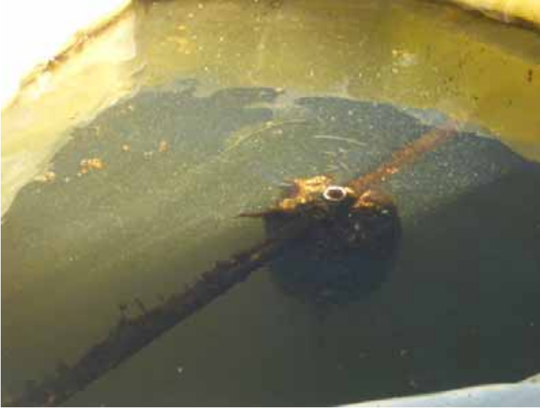
Figure 27. Condition of spreader axis and supporting float September 1. Note floating attached algae that had been dislodged from spreader assembly.
